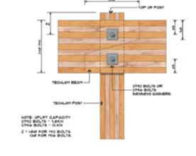
SCARF JOINT AT POSTS - FRONT VIEW (>240 DEPTH)
