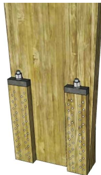
Figure 12. Quick-Connect Column to Foundation Connection
