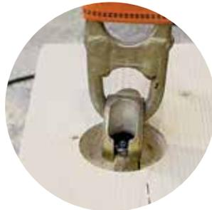
Lifting anchors used in combination with self-tapping screws, for lifting of solid timber beams or panels.
